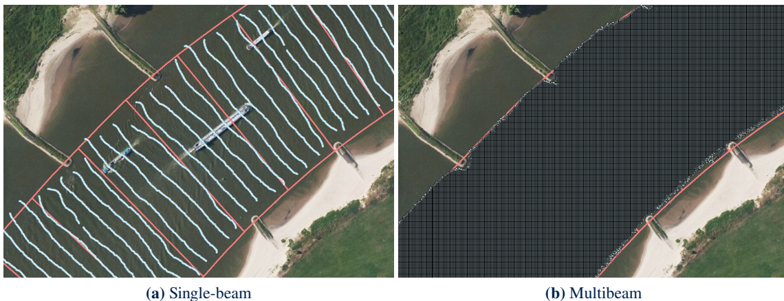
Figure 4: Spatial coverage of single-beam (year 1993) and multibeam (year 2011) echosoundings in the same section of the Waal (river km 880, upstream Nijmegen). The white dots and shaded areas indicate data points. The red rectangles are the surfaces in which the Rhine branches are subdivided. They are used to ensure that the same spatial domain is considered when comparing data from different years.
