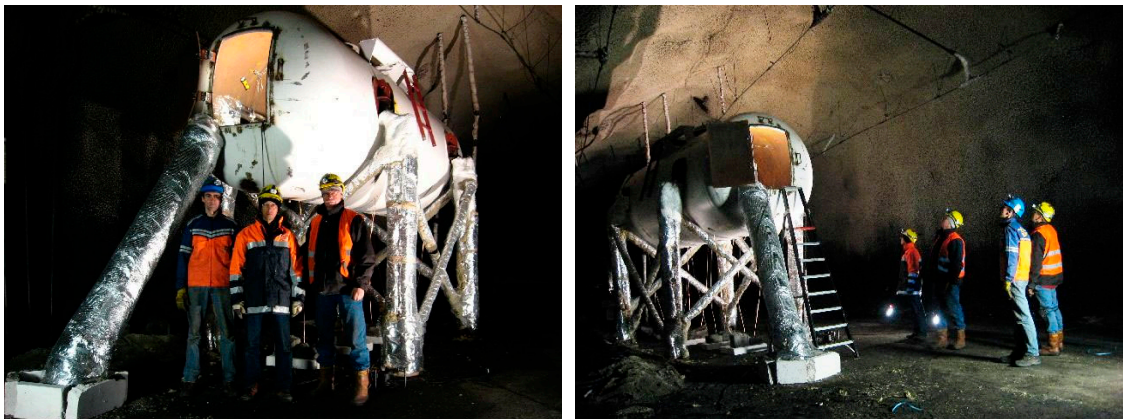
Figure 3.5 The actual test-tank after completing the installation in the Runehamar tunnel
