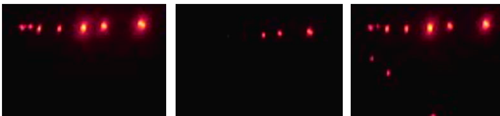
Stills from the video that were used to determine visibility. From left to right: before, during and after the test. Note the reflection of the beacons in the flooded road surface after the test.
