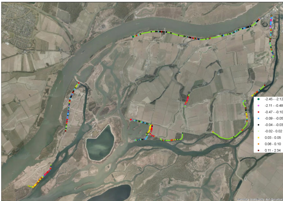
Figure 2.8 Comparison between the schematized kade heights and the measurements for the existing kades given as "As Built measured elevation – kade crest elevation"
