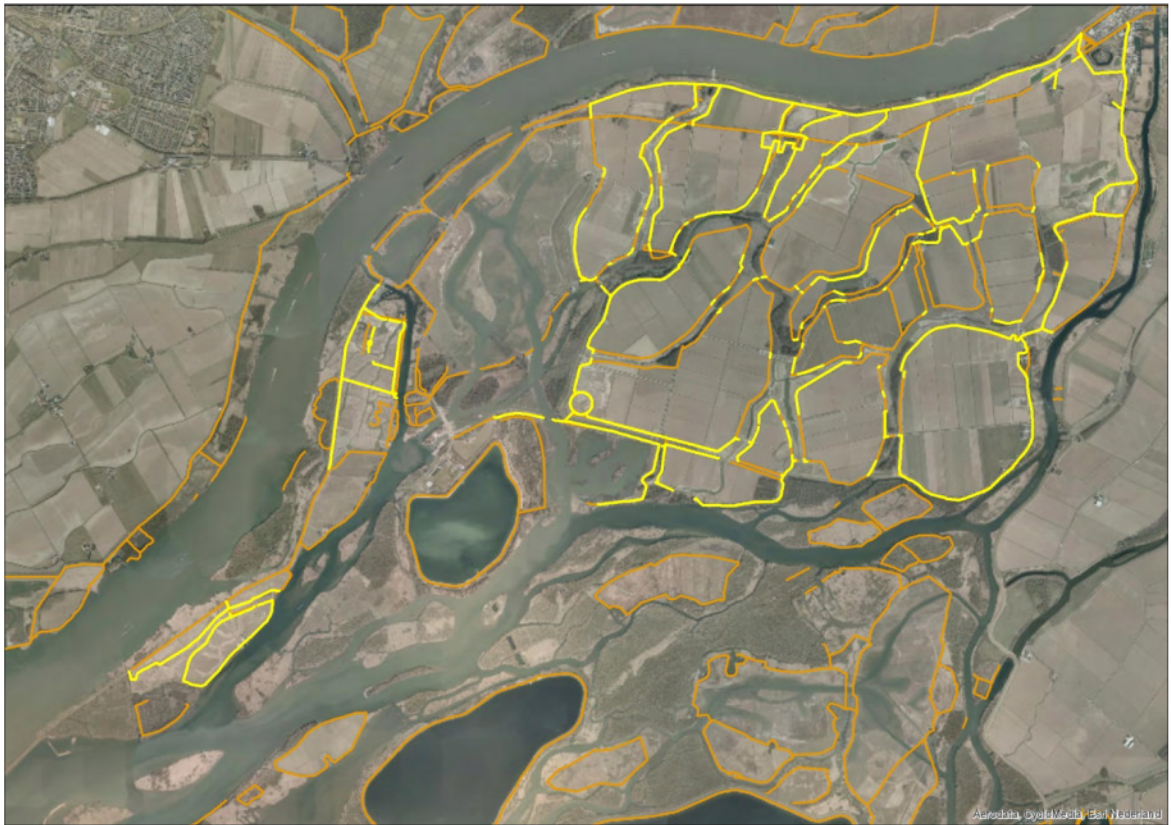
Figure 2.6 The locations (yellow line) where the kade position in the Eindontwerp variant slightly differs from the SNIP3 variant position (brown line). Background map: LuchtfotoNL 2013 (50 cm).
