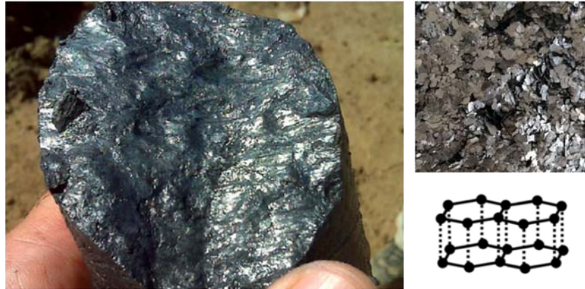
Figure 5 Natural flake graphite sample (left) and cross-section (top-right) along with the crystal structure (bottom-right). Source: Next Source Materials; Indiamart.
