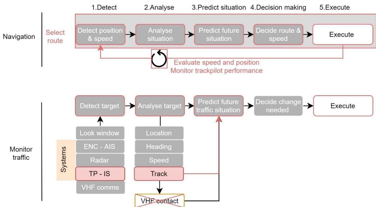
Figure 7 Changes to navigation tasks with IS
