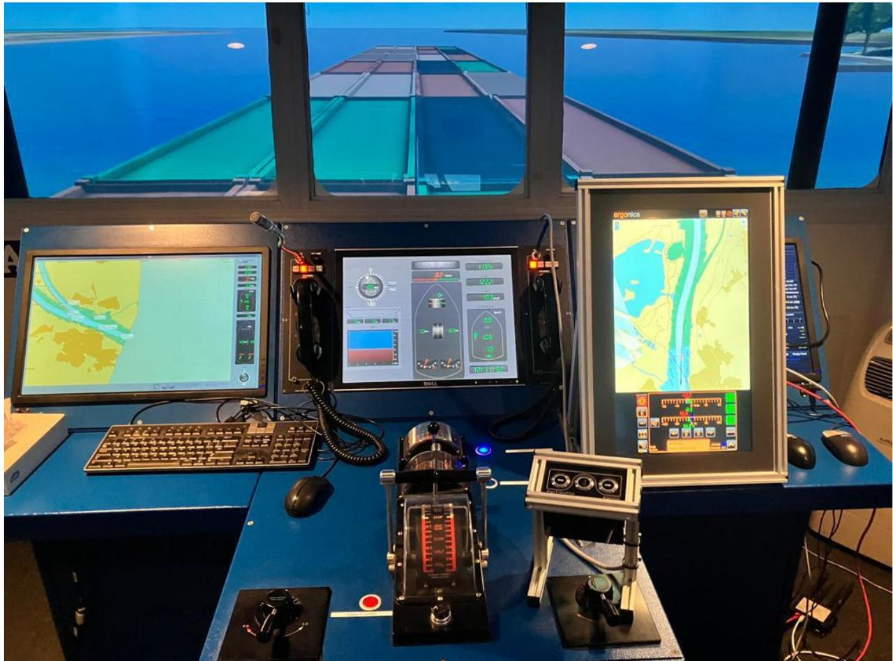
Figure 35 Simulator FMB2 with the trackpilot from Argonics
