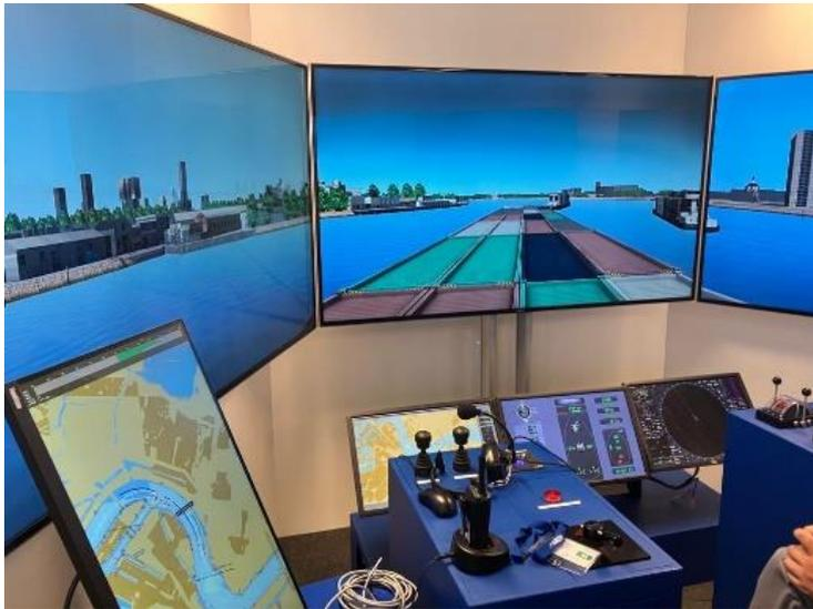
*Figure 1 Multi-purpose simulator with a trackpilot installed*
