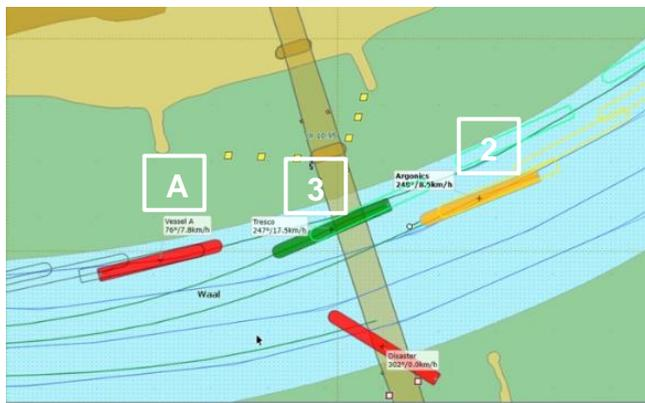
Figure 21 Still from simulation: vessel 3 (green) squeezes between vessel 2 (yellow) and vessel A (red).
