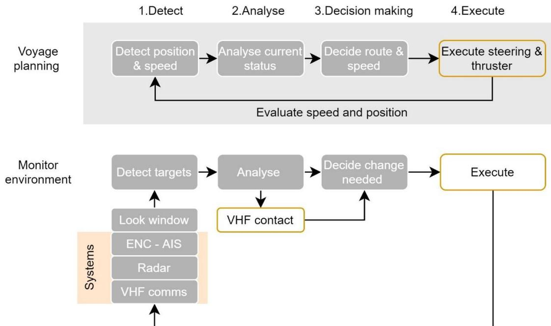
Figure 6 Task analysis navigation tasks
