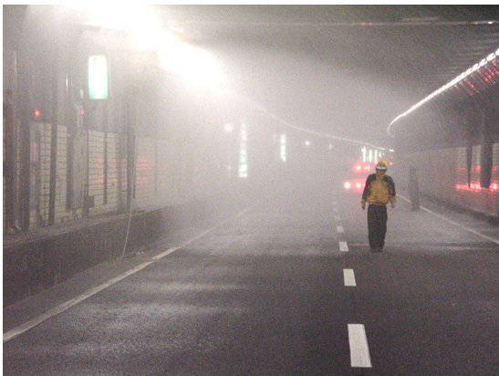
Figure D-27 Water spray
