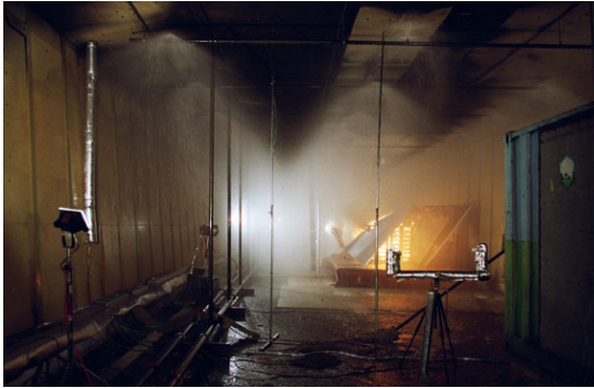
Test 12 load cabin cooled down by sprinkler
