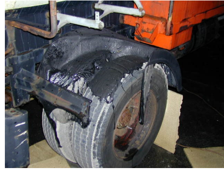
Test 14 wheel and plastic mud guard of tanker
